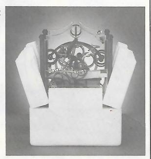
Carefully remove top foam and cut tape holding side pieces front and back. Remove side pieces of foam as seen in photo using care not to exert pressure inward.
